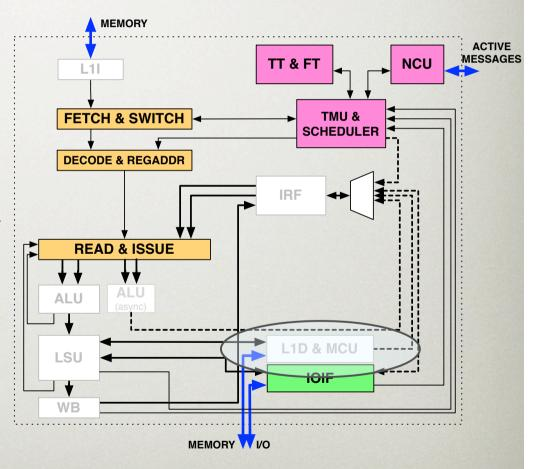
Upon completion of a longlatency operation (multi-cycle ALU, memory load) the value is written back asynchronously to the RF
