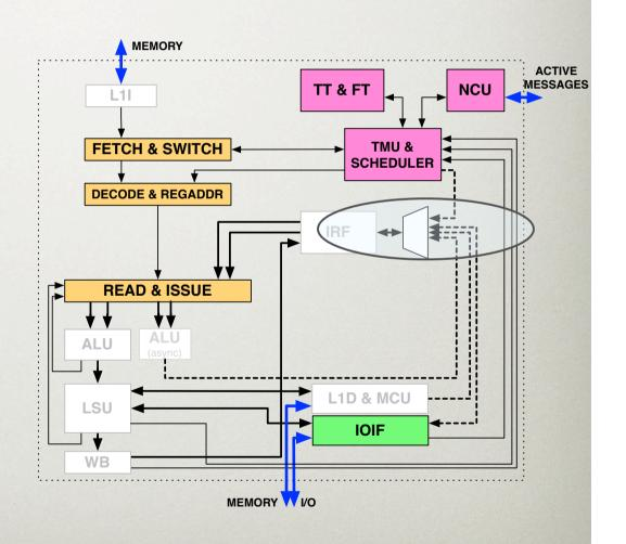
The Thread Management Unit handles thread creation, synchronization, and provides thread metadata to the pipeline
