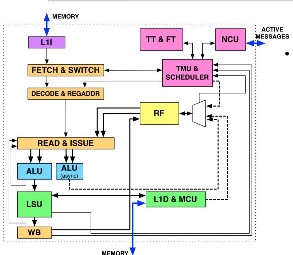
D-RISC cores: hardware multithreading + dynamic dataflow scheduling
