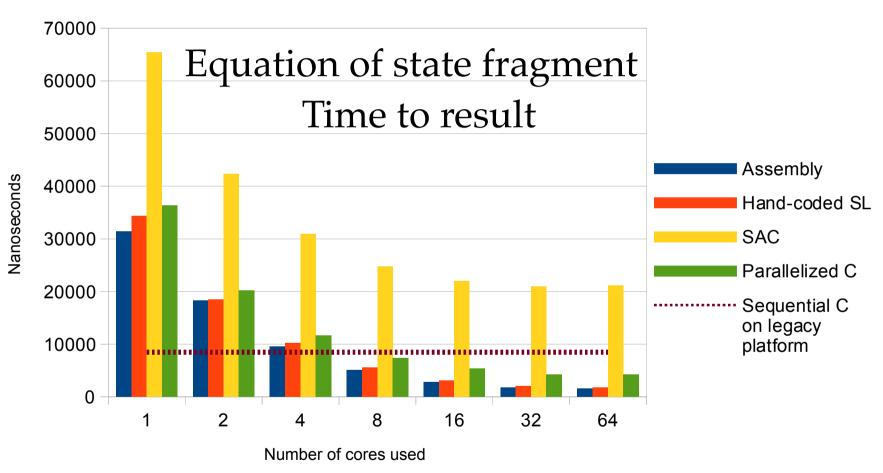
Legacy platform = MacBook Pro, Core 2 Duo @ 2.4GHz area(1 Core 2 Duo core) ~ area(32 Microgrid cores)
